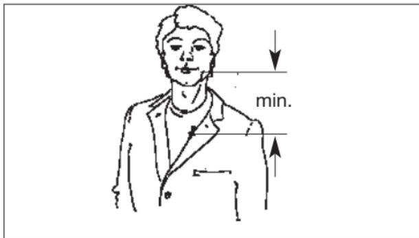
Fig. 6: Attaching the microphone near the user's mouth.
